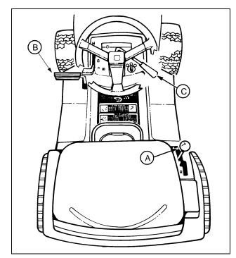
Move shift lever (A) to the right and forward to desired FORWARD speed.
